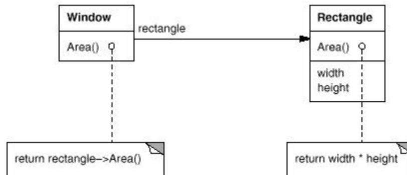
A plain arrowhead line indicates that a class keeps a reference to an instance of another class. The reference has an optional name, "rectangle" in this case.
