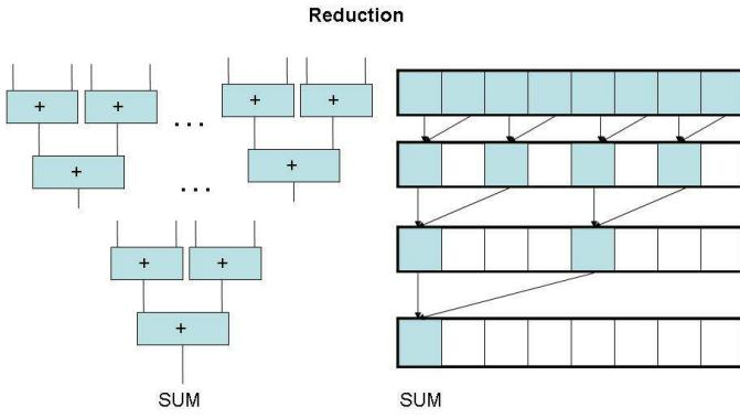
Fig. 1. Reduction on an FPGA and a GPU
