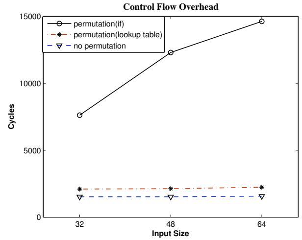
Fig. 2. Overhead of control flow in our CUDA implementation of DES.
