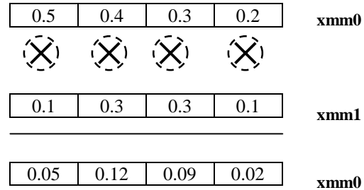
Figure 3: Example of the "mulps xmm0, xmm1" instruction
