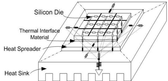
**Figure 3: Example compact thermal model with  $3 \times 3$  grid cells for silicon die [3]. For clarity of drawing, the structure is upside-down compared to the primary heat transfer path in Fig.1. Thermal capacitors and heat sources are also omitted for clarity.**
