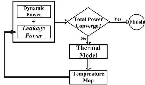
**Figure 2: A full-chip thermal model closes the loop for accurate leakage power calculations. The loop is iterated until either power/temperature convergence is achieved or thermal runaway is detected.**
