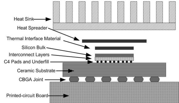
Figure 1: Packaging components in a typical CBGA package.
