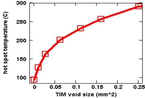
**Figure 7: The impact of the size of void defect in thermal interface material (TIM) to silicon die hottest temperature. Temperatures are normalized to the ideal case where there is no void defect in the TIM layer. TIM void sizes are with the unit of mm<sup>2</sup>.**
