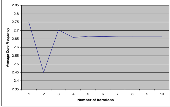
Figure 3. Average core frequency as the number of iterations in delay-thermal loop increases
