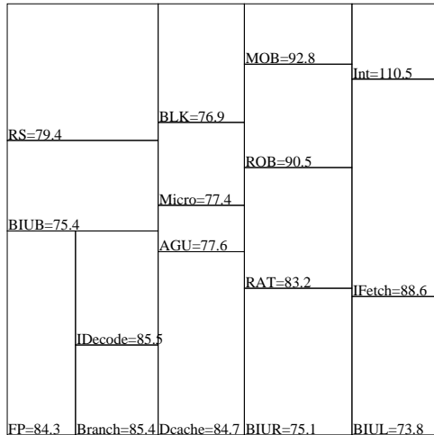
Figure 18: Pro-high: a floorplan with high maximum temperature for Pentium Pro
