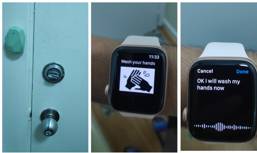
Figure 7: iWash implementation, with the beacon fitted at the door, user receiving reminder on the smartwatch and responding via voice interaction.
