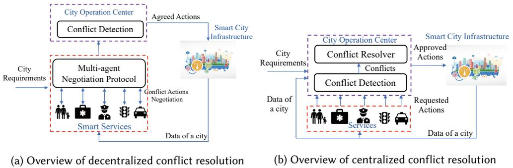
Fig. 2. Comparison of centralized and decentralized conflict resolution
