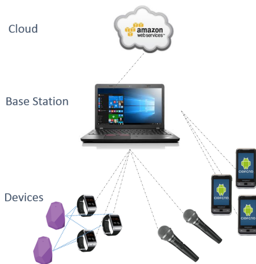
Fig. 1: Major Components of Residential Monitoring Systems
