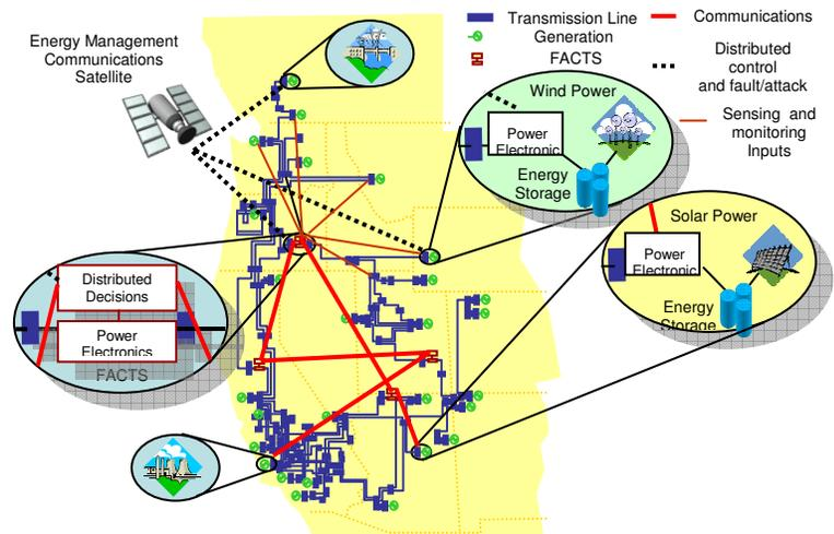
of the Electric Power Transmission Grid, Distributed Energy Resources (insets), and Cyber Coordination and Protection, which uses distributed decisions to coordinate control and system sensing to maintain correct operation, and to detect and react to faults and attacks.
