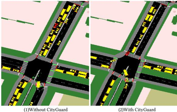
**Figure 6: Performances of traffic at the intersection between Bowery and Kenmare with and without CityGuard. Yellow and red objects denote regular and emergency vehicles. With CityGuard, there are higher traffic flow, less congestion, and emergency vehicles are prioritized for faster travel time.**
