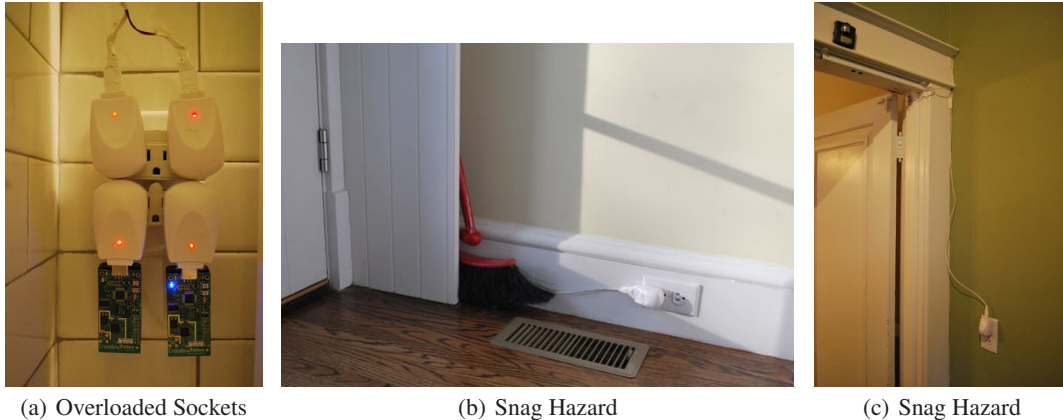
Figure 5. Wires are hazardous for reliability and maintenance. Users unplug devices when sockets are overloaded (a), and wires are often snagged, especially when they are near moving objects (b) or run through doorways (c).
