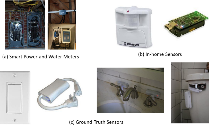
Figure 4: Our deployments included 25-40 sensors per home, including (a) a smart power and water meter (b) a motion and light sensor in every room. For experimental ground truth, we also deployed (c) Z-wave light switches, Z-wave plug load meters, and Z-wave contact switches on the water fixtures.
