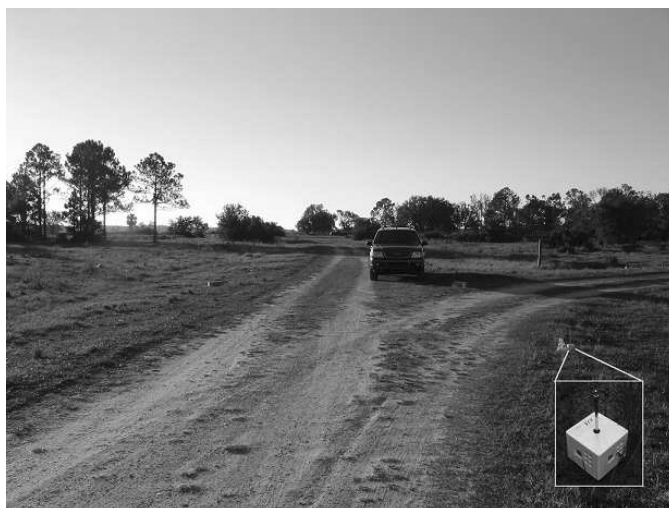
Fig. 10. Location of deployment and a deployed XSM mote. Nodes are randomly placed roughly 10 meters apart, covering a 300-meter road that intersects a 200-meter road.
