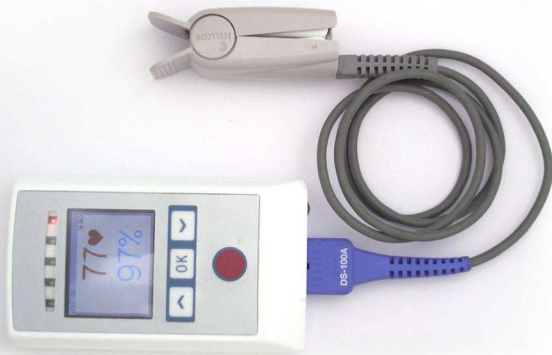
Fig. 2. Medical information tag, or miTag for short, used in MEDiSN [42]. The miTag is a Tmote mini [52] based patient monitor that includes a pulse oximetry sensor with LEDs, buttons and a LCD screen. The miTag is powered using a re-chargeable 1,200 mAh 3.7 V Li-Ion battery and external finger tip sensors are used to make the pulse oximetry measurements.
