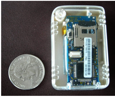
Fig. 1. The SHIMMER wearable sensor platform. SHIMMER incorporates a TI MSP430 processor, a CC2420 IEEE 802.15.4 radio, a triaxial accelerometer, and a re-chargeable Li-polymer battery. The platform also includes a MicroSD slot supporting up to 2 GBytes of Flash memory.
