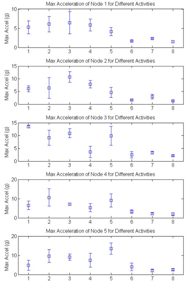
**Figure 7: The max acceleration of nodes for different activities: 1) fall forward; 2) fall backward; 3) fall leftward; 4) fall rightward; 5) stumble and fall; 6) walk; 7) sit down; 8) lie down.**
