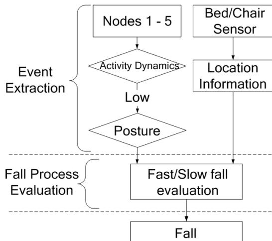
**Figure 2: The main process to detect falls: posture recognition, localization, and fall process evaluation for both fast and slow falls.**
