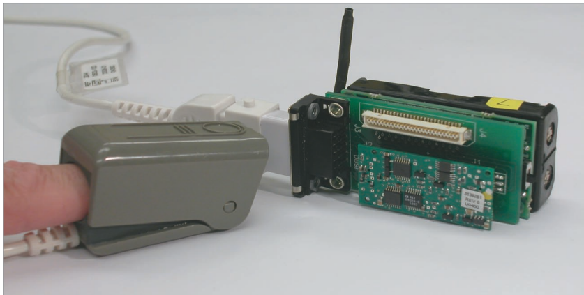
Figure 4. Pulse oximeter measures blood oxygen levels and is connected to a smart sensor node similar to the one shown in Figure 1.
