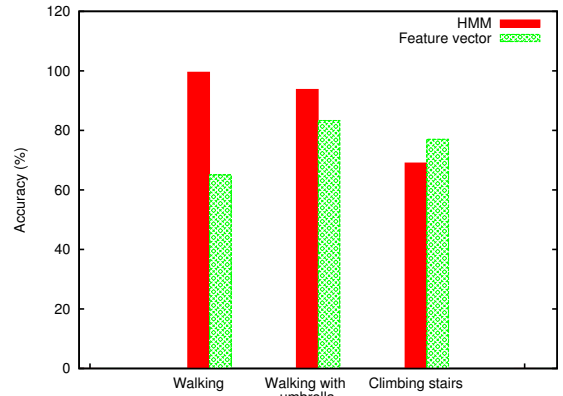
Figure 16: Accuracy of non-stationary activity identification using HMMs and feature vectors
