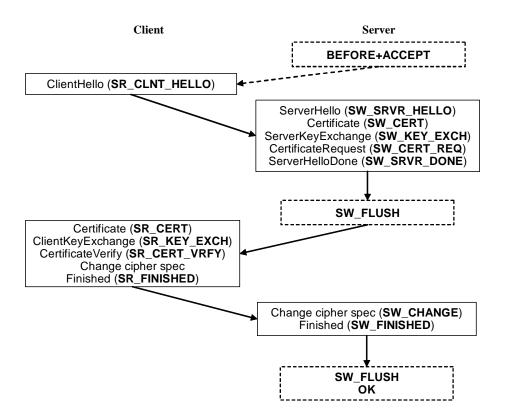
FIGURE 8.27: SSL handshake protocol states.
