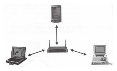
**Figure 2.1** Basic service set architecture illustration [9]. The double pointed arrow indicates two-way communication between any of the devices. The access point is the device in the middle, connected wirelessly to a PDA, a laptop, and a desktop computer.
