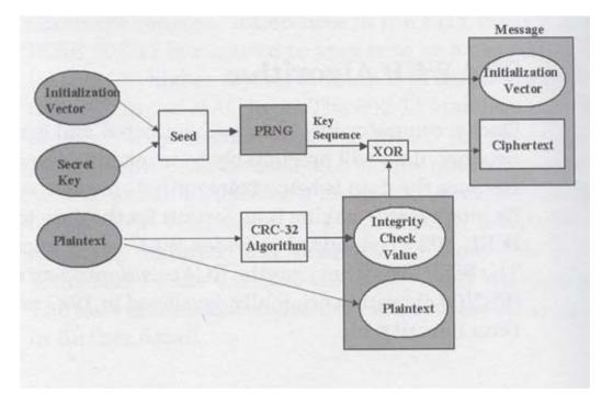
**Figure 3.2** WEP Decryption [13]. The WEP encryption process starting with the plaintext, secret key, and the initialization vector to the final cipher text and generated frame. The act of concatenating the initialization vector, followed by the MAC protocol data unit, followed by the integrity check value generates the frame body.
