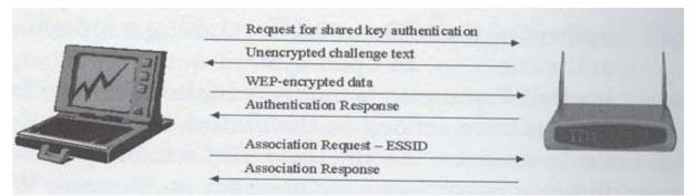
**Figure 3.3** Authentication and Association Process[10]. The authentication and association process starts by the client sending a request for a shared key authentication. The authentication process completes when the client passes the unencrypted challenge text. The association process then starts with the client sending its ESSID. The whole process completes when the access point replies with the association response.
