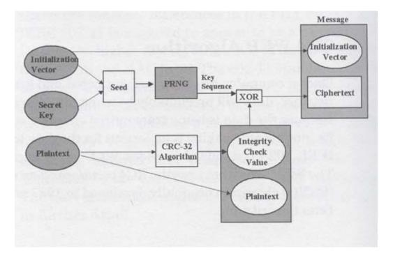
**Figure 3.1** WEP Encryption [13]. The WEP encryption process starting with the plaintext, secret key, and the initialization vector to the final cipher text and generated frame. The act of concatenating the initialization vector, followed by the MAC protocol data unit, followed by the integrity check value generates the frame body.
