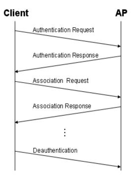
**Figure 4.1** Graphical depiction of the normal authentication process (Created by Author). The Client begins by sending its authentication request to an access point. The omitted (...) part indicates data transferred. The deauthentication message at the end can go in both directions.
