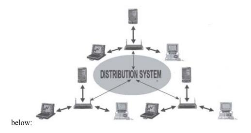
**Figure 2.2** Extended service set architecture [9]. Three basic service sets shown here are connected to the distribution system (DS). The DS is a logical concept. It is independent of the media connecting an access point to another element of the distribution system.
