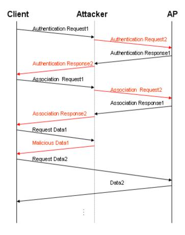
**Figure 4.2** Graphical depiction of the PiM attack (Created by Author). Arrows marked in black are legitimate management messages. Arrows marked in red are messages generated by the attacker.
