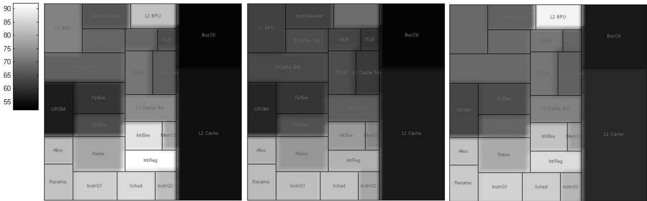
Figure 5. Hot spot movement. Hottest block moves from the integer register file to the scheduler unit, and then to the L2 BPU
