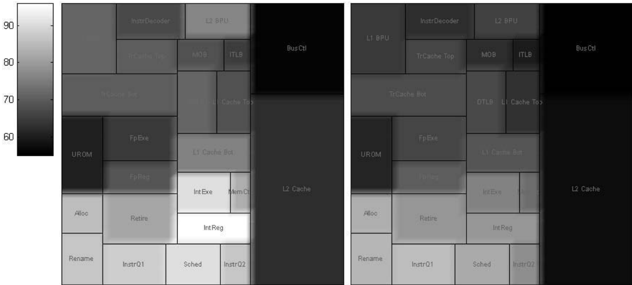
Figure 3. (a) Temperature change over time (gzip) (b) Temperature change over time (wupwise) and (c) Spatial difference for gzip and wupwise benchmarks
