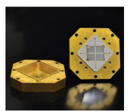
QUANTUM DEVICE: A circuit for measuring superconducting qubits is housed in a gold-plated box. These measurements can entangle qubits in separate clusters, or "modules," allowing modules to connect to form a unified quantum computer.
