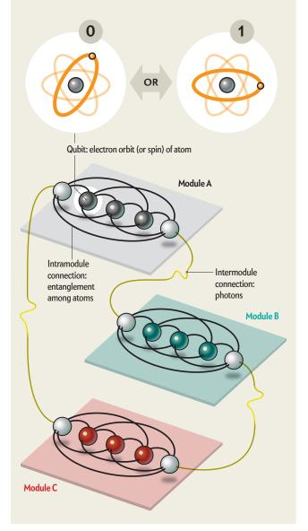
another through their electrical repulsion and can be confined with electromagnetic fields generated by nearby electrodes. We can laser-cool hundreds of trapped ions to form a stationary crystal of individual atoms that act like identical pendulums connected by springs. Additional control lasers can push the ions around in a way that can entangle their spin states through the vibrations of the ions, in a scheme first proposed in 1995 by
