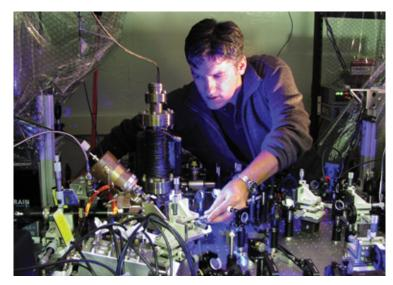
LAB WORK: Author Christopher R. Monroe manipulates atomic ion qubits with lasers and confines them in a trap made of electromagnetic fields generated by electrodes.
