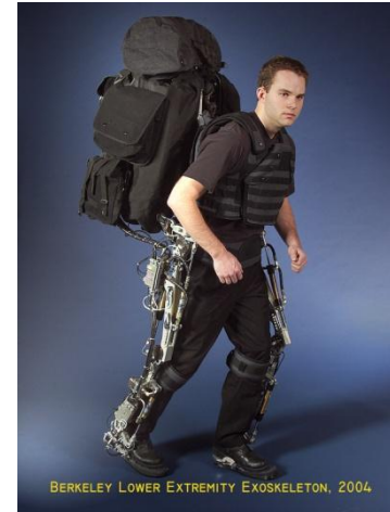
Berkeley Lower Extremity Exoskeleton 2004, can carry 150 lbs at 4 mph
