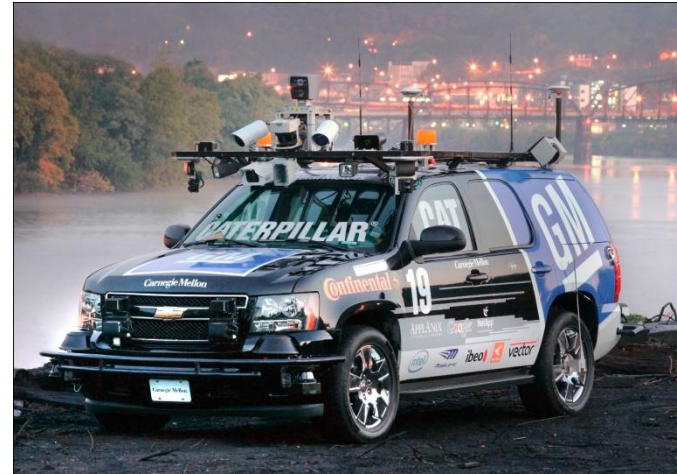
“Boss” autonomous vehicle, CMU navigated 60-miles in 4:10 hours first-place winner ($2 million) DARPA Urban Challenge, 2005
