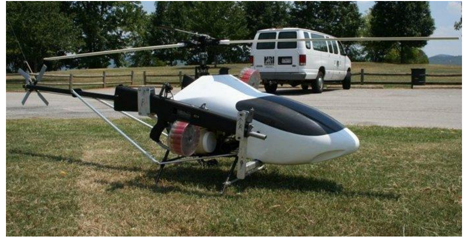
AutoCopter Gunship by Neural Robotics, Inc., 2006 (two MPS AA-12 automatic shotguns, high-explosive & armor-piercing rounds, 5 shots per second), cost: $200K
