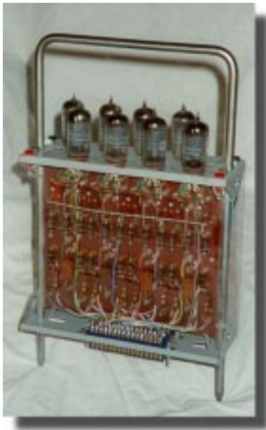
A single digit from the accumulator of a Burroughs 205, circa 1954. The 205 was a decimal machine with a magnetic drum for primary memory. This device, about the size of a modern laptop, stored one decimal digit (i.e., 4 bits!)
