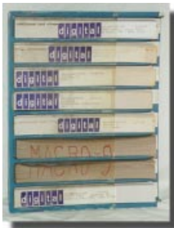
A "DEC tape" - a magnetic tape used on several early DEC computers. It was notable in that it was addressable: one could move forward or backward to a specified tape block. This particular tape contains the source code for the first Pascal Compiler, written by the inventor of Pascal, Nicklaus Wirth.
