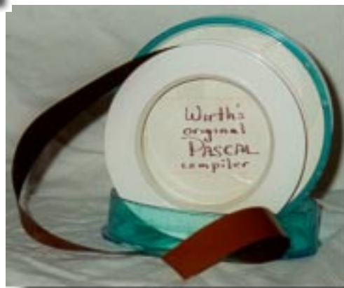
A "DEC tape" - a magnetic tape used on several early DEC computers. It was notable in that it was addressable: one could move forward or backward to a specified tape block. This particular tape contains the source code for the first Pascal Compiler, written by the inventor of Pascal, Nicklaus Wirth.
