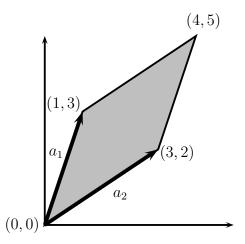
Figure 1: Illustration of the determinant for the  $2 \times 2$  matrix A given in (1). Here,  $a_1$  and  $a_2$  are vectors corresponding to the rows of A, and the set S corresponds to the shaded region (i.e., the parallelogram). The absolute value of the determinant,  $|\det A| = 7$ , is the area of the parallelogram.
