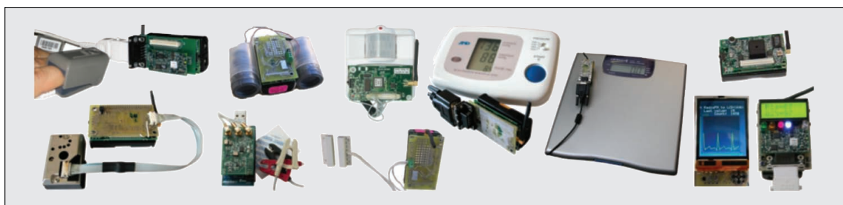
■ Figure 7. Sensor and display hardware in AlarmNet.
