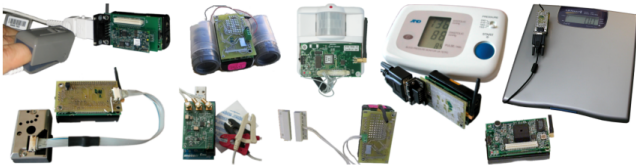
Figure 6: Sensor hardware supported by SenQ in AlarmNet.
