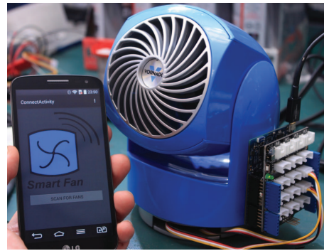
Fig. 6: 802.15.4 and BLE connected prototype smart appliance
