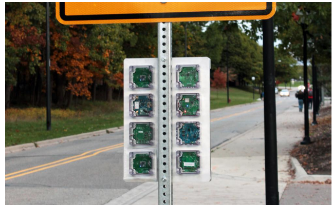
Figure 1: The Signpost platform easily mounts to existing street sign posts, harvests from an integrated 0.1 m 2 solar panel, and provides tenant sensor modules with power, communications, processing, storage, time, and location. Signpost is open source, with all hardware and software available online. †
