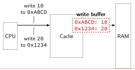
write appears to complete immediately when placed in buffer memory can be much slower
