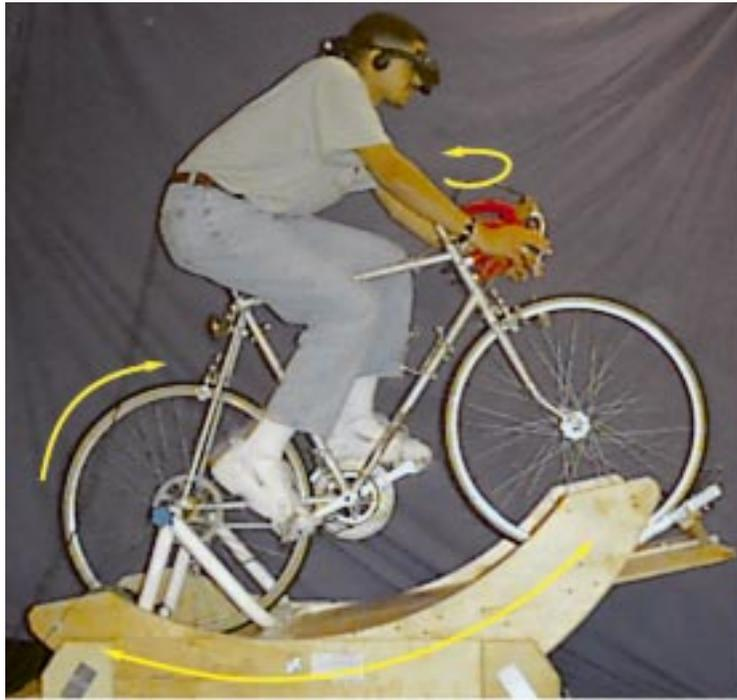
rear wheel. The connecting springs are two-sided, and the cyclist can pull up on the pedals as if the bicycle were equipped with toe-clips. The details of the bicycling control system appear in Hodgins et al.<sup>16</sup>
