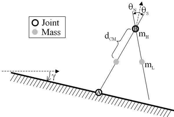
Figure 2: A bipedal walker. Lumped masses are positioned at the hip ( $m_H$ ) and on each leg ( $m_L$ ). The spacetime-constraints walker applies torques at the stance foot (A) and at the hip (B).
