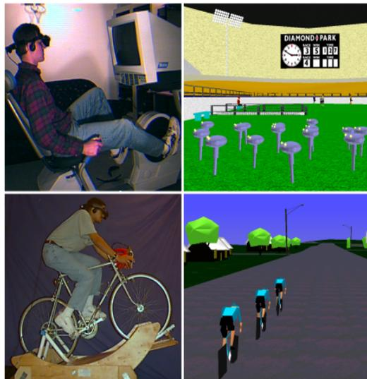
Figure 1: Images of a user on the Tectrix bike, the robot herding game, a user on the motion platform, and the Atlanta Road Race course environment.
