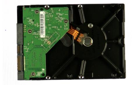
Where our DRAM was two gigabytes, this hard drive can store one terabyte, which is 500 times as much memory. A terabyte is close to a trillion bytes:
