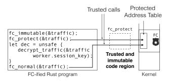
Figure 2: The trusted region is an address (in the code of FC's user space library) to which calls from mprotect must return to, which is ensured by FC's kernel module. The kernel module traps and monitor all calls to mprotect and maintains a list of page addresses in the protected address table for each thread.
