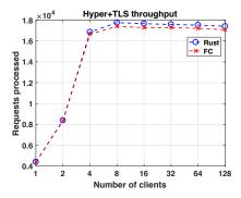
Figure 5: Throughput of a Hyper server using Rust TLS in 60 seconds. Requests are sent locally using  $2^k$  threads for  $k \in [0,7]$ .
