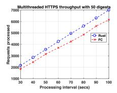
Figure 4: Throughput of an openss1 HTTP in 30–100 seconds. Each request has 50 calls to ring's digest. In the FC-enabled server, each digest iteration creates and releases a secure compartment.
