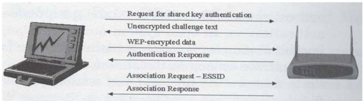
**Figure 3.3** Authentication and Association Process[10]. The authentication and association process starts by the client sending a request for a shared key authentication. The authentication process completes when the client passes the unencrypted challenge text. The association process then starts with the client sending its ESSID. The whole process completes when the access point replies with the association response.
