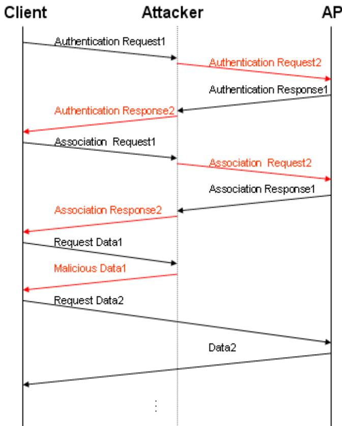
**Figure 4.2** Graphical depiction of the PiM attack (Created by Author). Arrows marked in black are legitimate management messages. Arrows marked in red are messages generated by the attacker.
