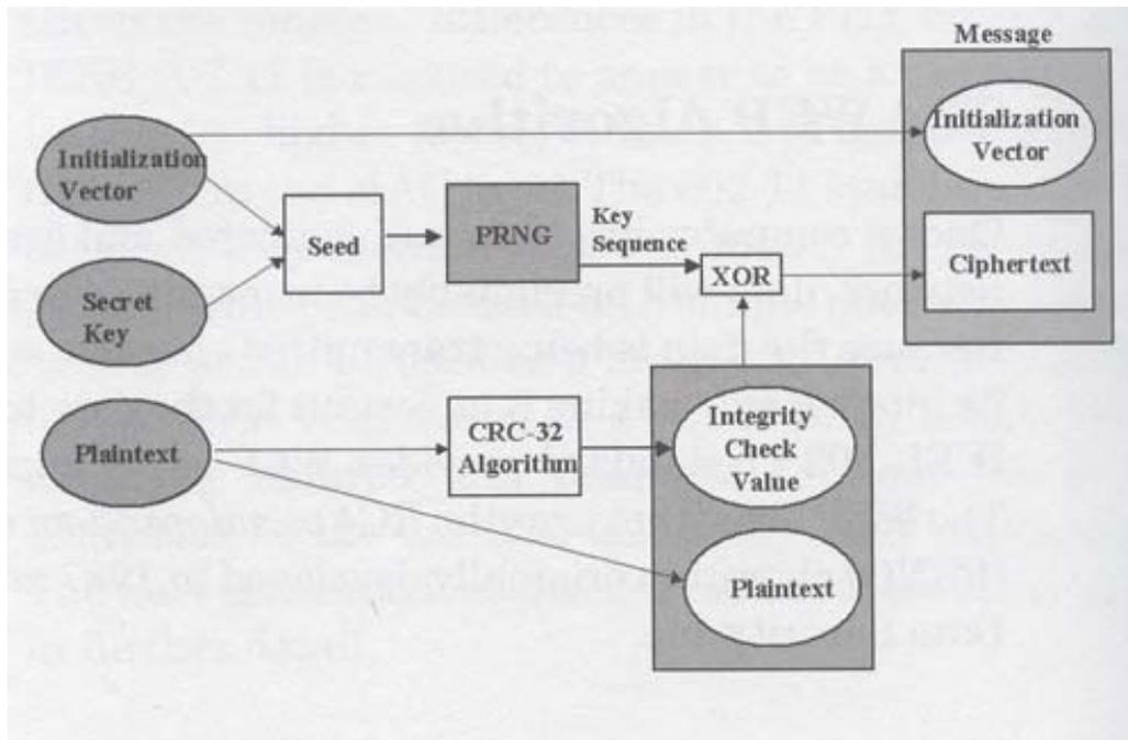
**Figure 3.2** WEP Encryption [13]. The WEP encryption process starting with the plaintext, secret key, and the initialization vector to the final cipher text and generated frame. The act of concatenating the initialization vector, followed by the MAC protocol data unit, followed by the integrity check value generates the frame body.
