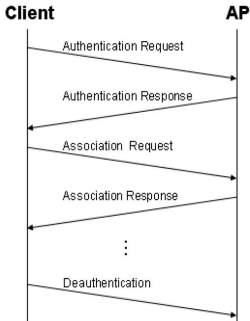
**Figure 4.1** Graphical depiction of the normal authentication process (Created by Author). The Client begins by sending its authentication request to an access point. The omitted (...) part indicates data transferred. The deauthentication message at the end can go in both directions.
