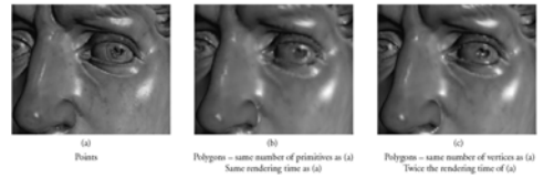
Figure 5: Comparison of renderings using point and polygon primitives.
