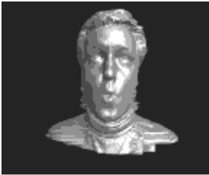
Plate 1. The model for the “PLB Head” test case (59,592 polygons). As in the National Computer Graphics Association Graphics Performance Committee’s Program Level Benchmark, the model rotates 360 degrees about a vertical axis in 4.5 degree increments. The model is courtesy of the IBM AWD Graphics Lab, Austin, Texas.
