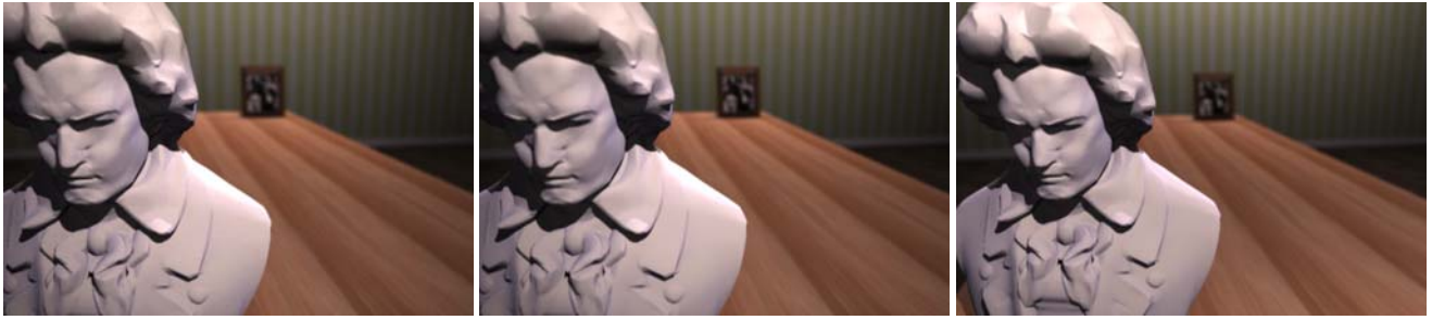
Figure 9: Images synthesized with a 35mm wide-angle lens using, in order of decreasing accuracy, the full lens simulation (left), thick approximation (center), and the standard model (right). The top left arrow indicates the location of the scanline used in Figure 11.
