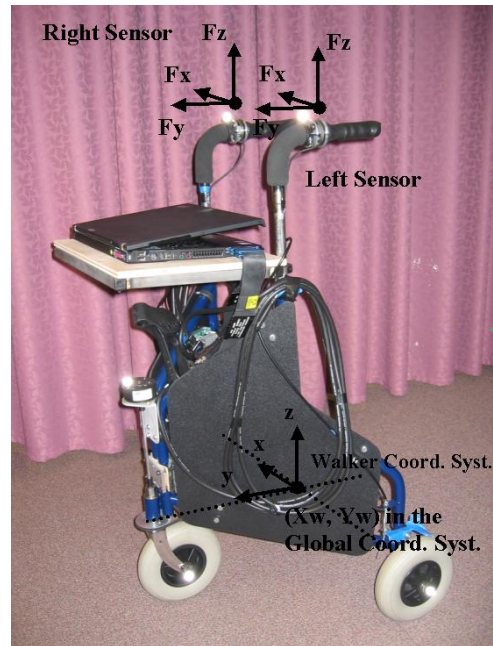
Figure 3. Walker with Handle Axes for Force and Moment Components
