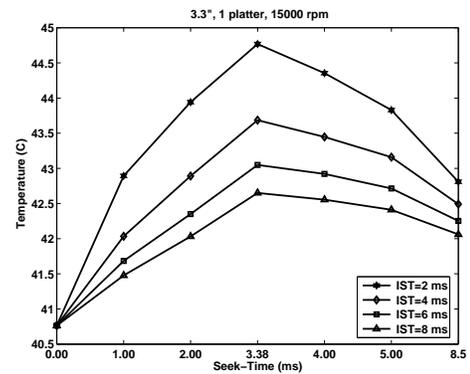
Figure 6: Relationship between seek-time and disk temperature for a 1-platter 15K RPM disk drive.
