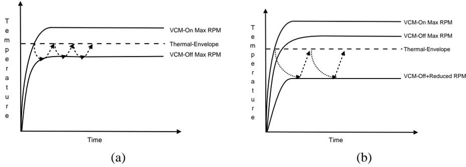
Figure 4: Dynamic Thermal Management techniques. In (a), temperature control is achieved by modulating movement of the disk arm. In (b), RPM modulation is employed.
