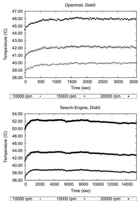
Figure 3: Thermal profiles of the applications.
