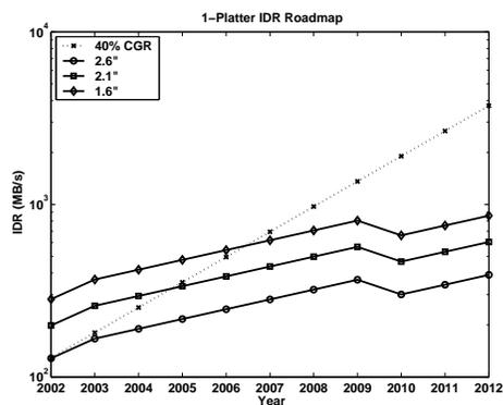
Figure 1: Disk Drive Roadmap. Each solid curve gives the maximum attainable IDR within the thermal envelope. The dotted line indicates the 40 percent target growth rate in IDR.
