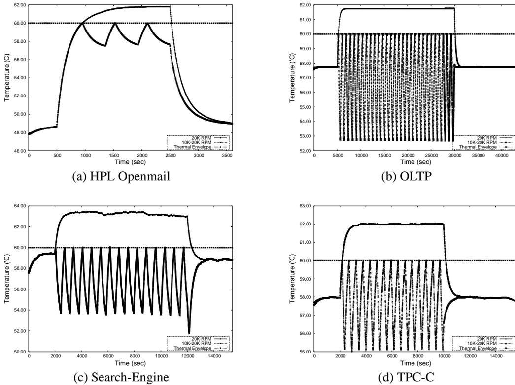
**Figure 3.** Thermal profiles of the real workloads for  $DRPM_{opt}$  under the scenarios of Table 1. They are all for the disk0 of disk arrays each of which is a 10K-20K multi-speed disk with 7 seconds of RPM transition time and 400 seconds of a cooling unit time.
