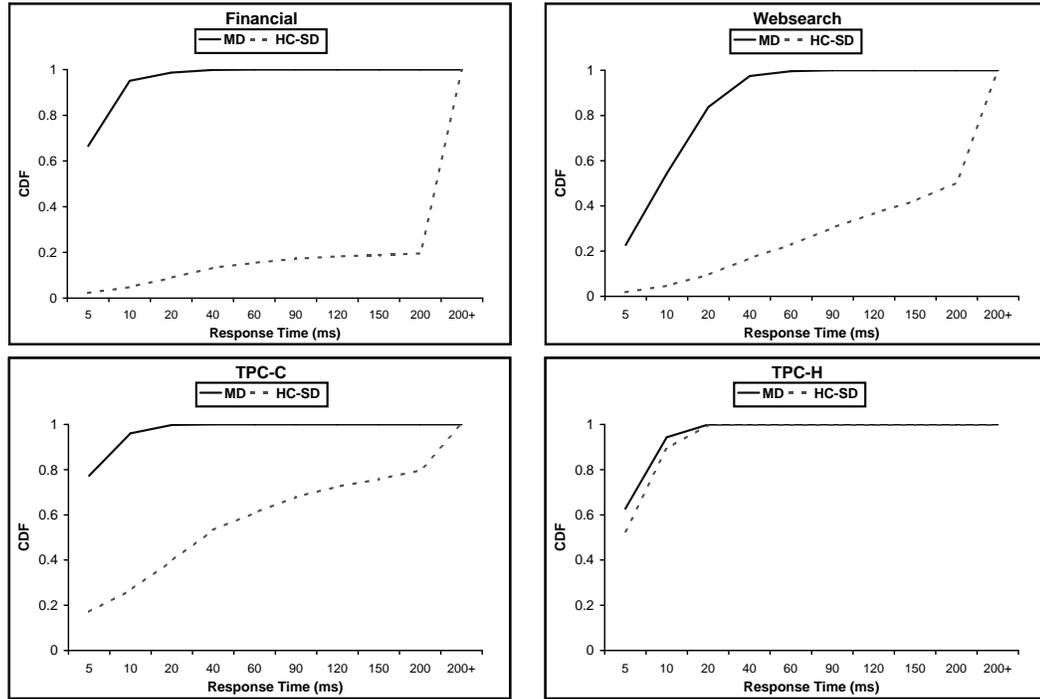
Figure 4.1: The performance gap between *MD* and *HC-SD*.
