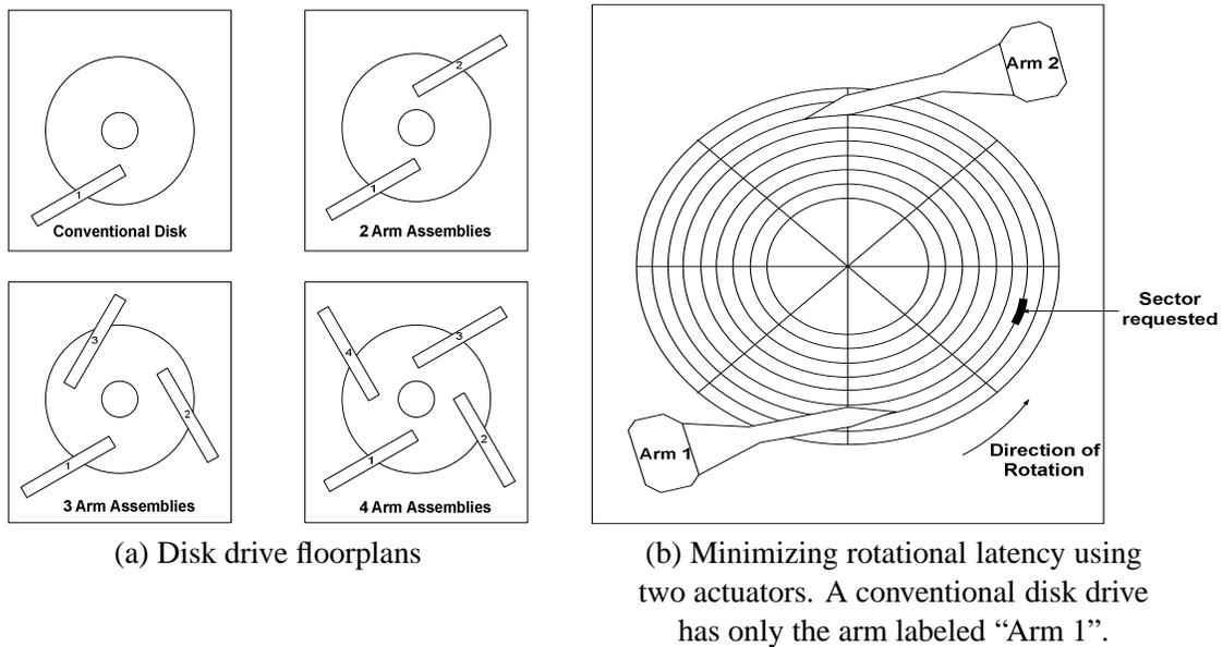
Figure 4.4: Intra-disk parallelism along the  $A$ -dimension.
