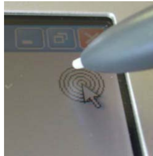
Figure 1. The distance between the pen tip and the actual screen creates a parallax that can amount to 15 pixels or more. So, controls and hotspots should be made large.
