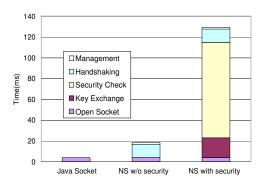
Figure 4: Breakdowns of the latency to open a connection.
