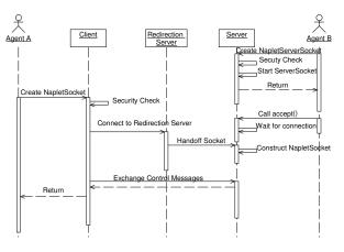
Figure 3: Socket handoff in connection setup.
