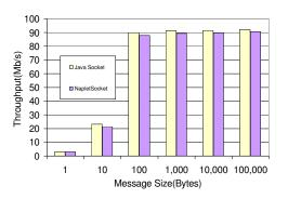
Figure 5: Throughput of NapletSocket vs. Java Socket.
