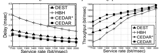
Fig. 11. Packet delay and throughput (with OPTIMAL).
