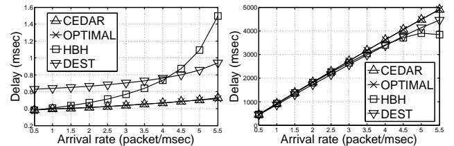
Fig. 10. Packet delay and throughput.
