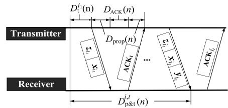
Fig. 3. Transmission and propagation delay.
