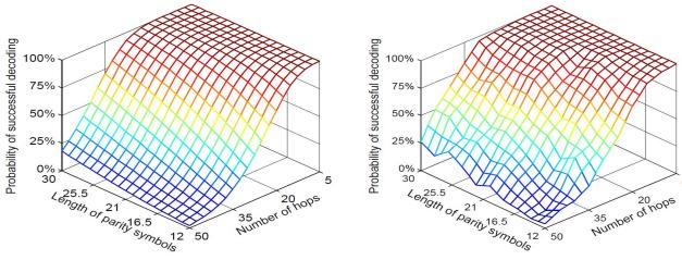
(a) The surface of  $F_\alpha(n, m_i)$  (b) Simulation results
