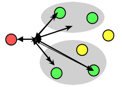
Incast is a many-to-one communication pattern commonly found in cloud data centers. It begins when a singular parent server places a request for data objects to a large number of servers simultaneously.
