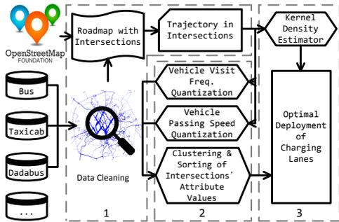
Fig. 6: Framework of CatCharger.
