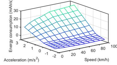
Fig. 3. Energy consumption of a pure EV (where  $\theta = 0$ ).
