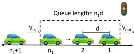
Fig. 1. A vehicle queue in front of a traffic light.
