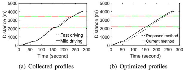
Fig. 8. Total driving time of different velocity profiles.
