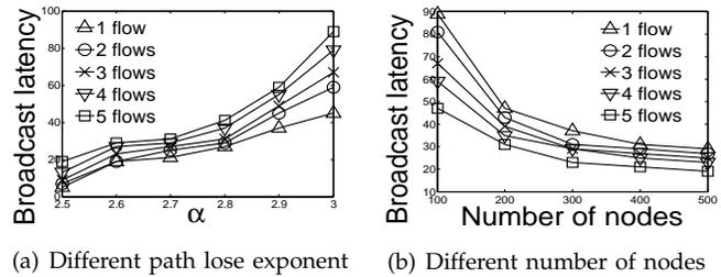
Fig. 9. Broadcast latency of PCBH in multi flow case with different number of flows
