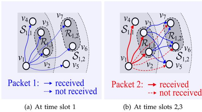
Fig. 3. An example of serial transmission
