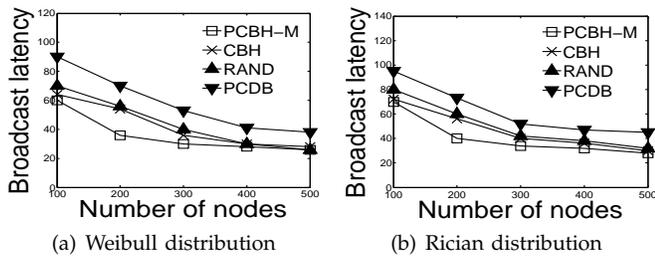
Fig. 8. Broadcast latency in multi-flow case under different fading models
