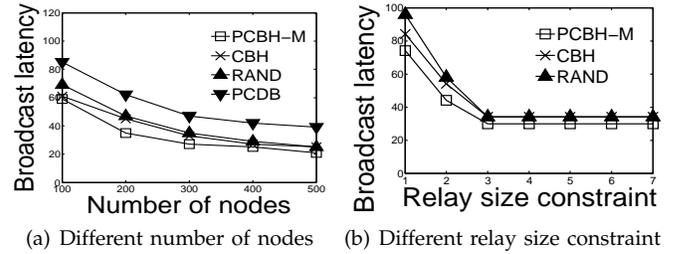
Fig. 6. Broadcast latency in multi-flow case with different number of nodes and different relay size constraint
